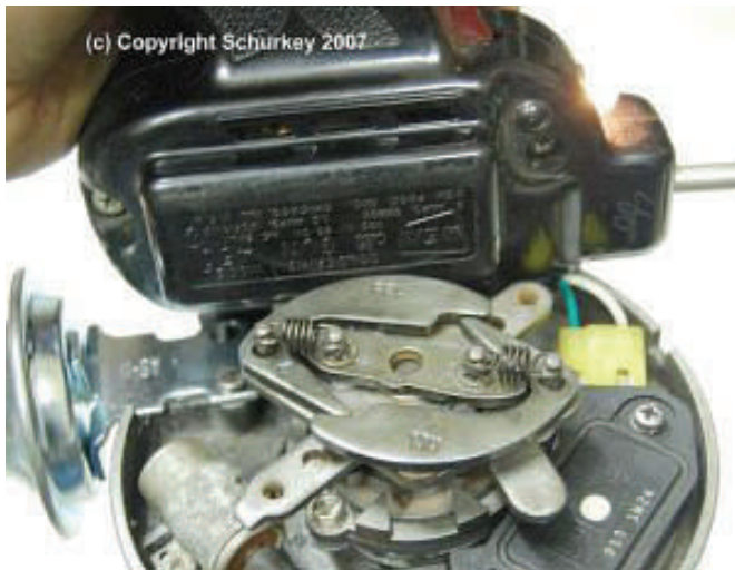
Photo 12. Using soldering gun to induce voltage into pickup coil.
