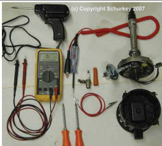
Photo 7. The tools you need to diagnose an HEI that has a 4-terminal module. (cranking buddy not shown—see "Victoria's Secret" catalog models for suggestions for a helper.)
